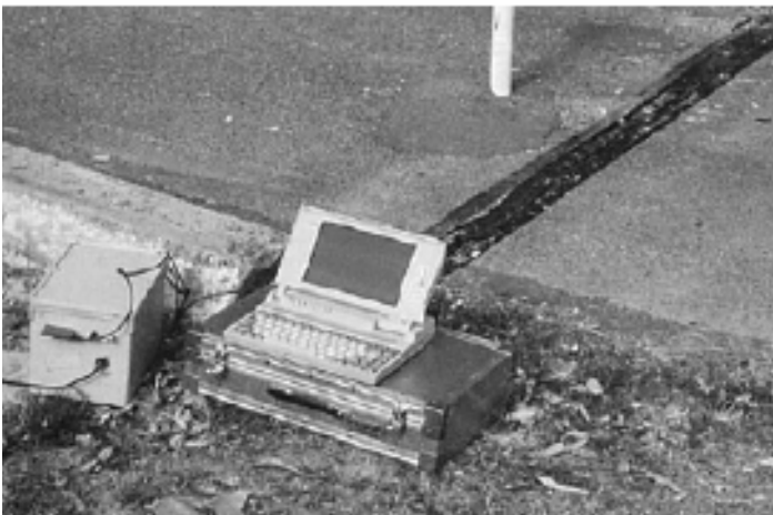
Figure E 3: Downloading data from a bicycle counter
