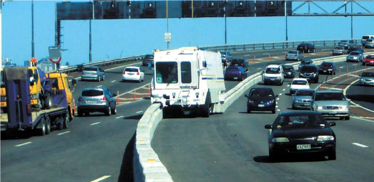
Figure 7.2: Concrete barrier moveable median
