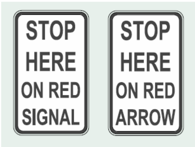
Figure 8.46: Stop here on red signal (R6-6) and stop here on red arrow (R6-14) signs
