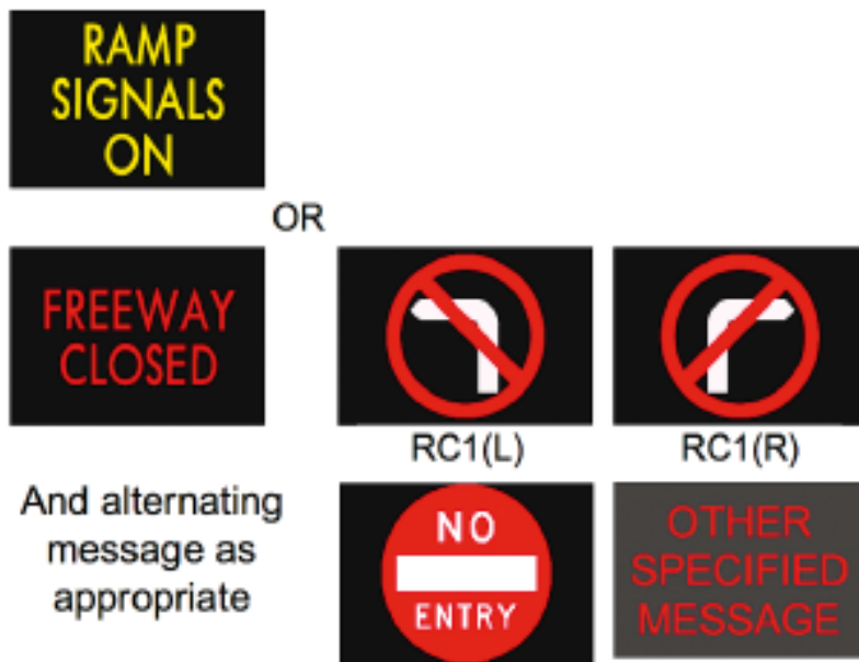
Figure 5.8: Example of electronic ramp control sign messages
