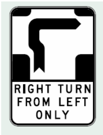
Figure 8.54: Hook turn sign
