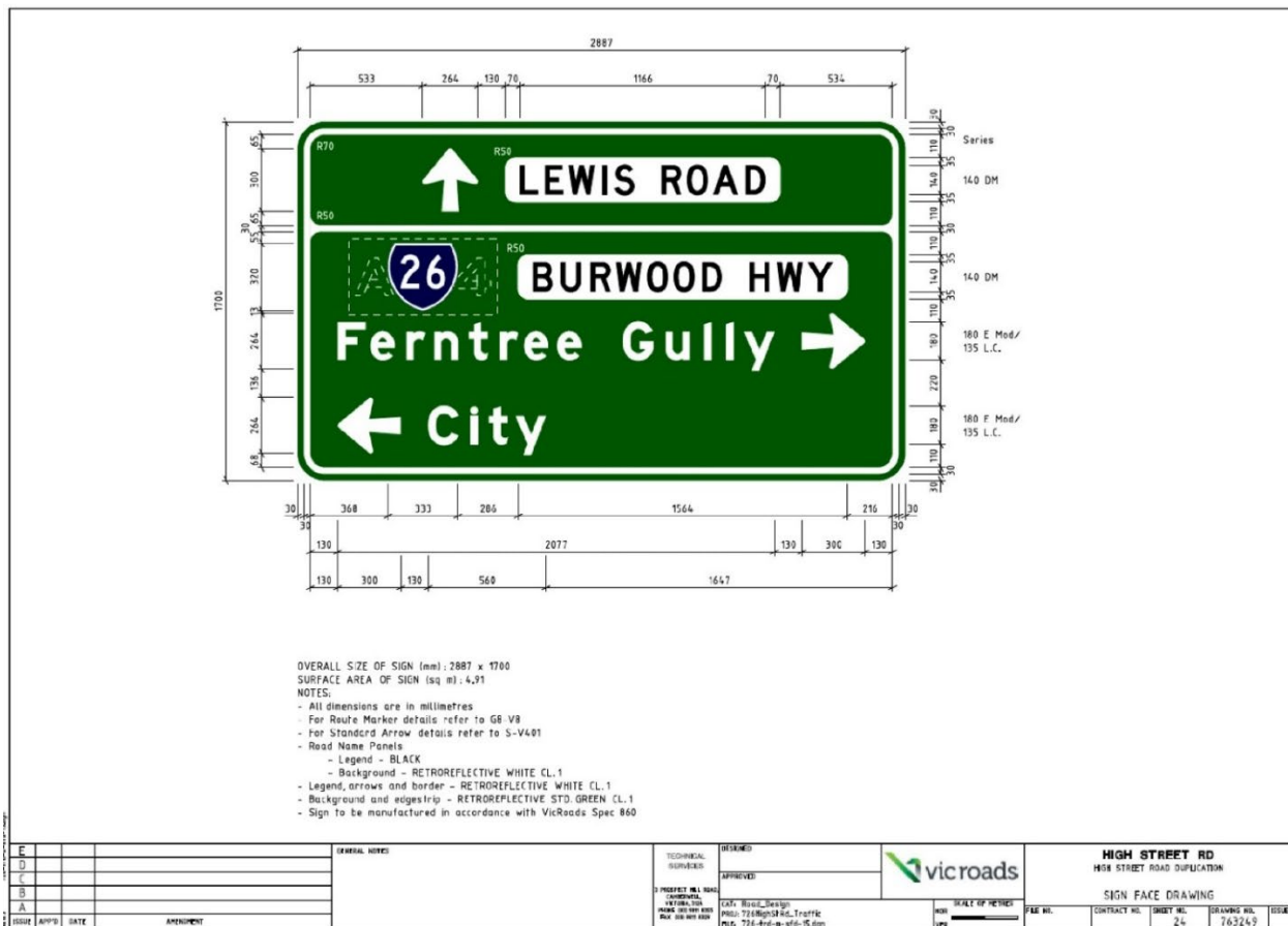
Figure 4.2: An example of a drawing for a made-to-measure intersection direction sign (G2-1)
