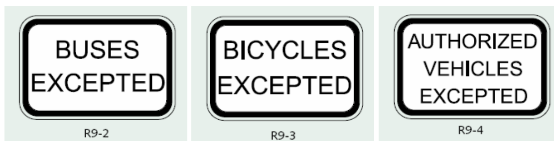
Figure 8.51: Supplementary plates exempting special vehicles from turn bans
