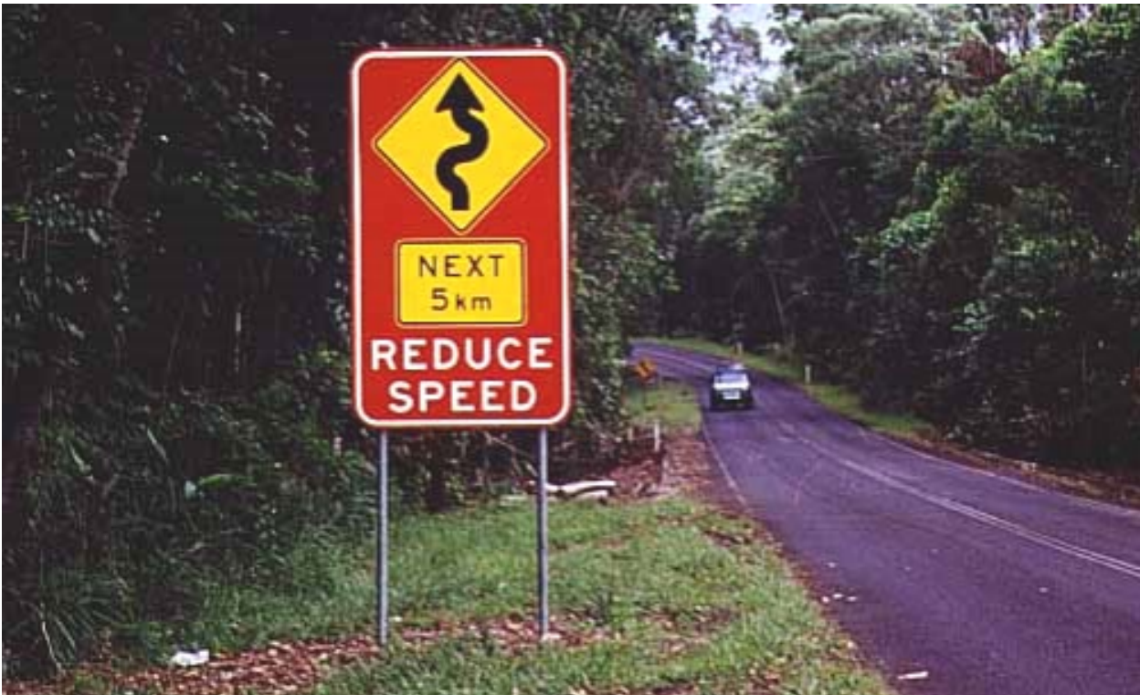
Figure 4.1: Red background used to emphasise a potential hazard
