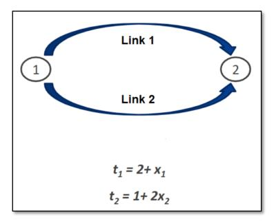
The figure above shows two unidirectional links (roads) connecting the Origin (Point 1) and the Destination (Point 2). The equations shown in the figure represent the link cost functions, i.e. the relationship between travel time in minutes (denoted  $bt_iy$ ) and the traffic flow in vehicles per hour (denoted by  $x_i$ ) on a link (denoted by i).
